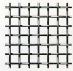
6 x 6 mesh .035" diameter wire; .132" opening
