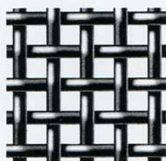
4 x 4 mesh; .080" diameter wire; .170" opening
