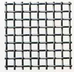
8 x 8 mesh .028" diameter wire; .097" opening
