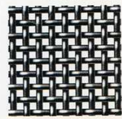
8 x 8 mesh; .063" diameter wire; .062" opening
