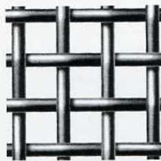
3 x 3 mesh; .105" diameter wire; .228" opening
