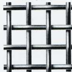
3 x 3 mesh .063" diameter wire; .270" opening
