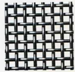
8 x 8 mesh; .047" diameter wire; .078" opening
