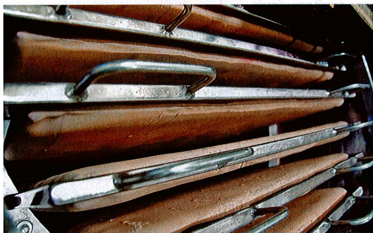
▶ The filter leaves at Royal Wine were redesigned by Newark Wire Cloth. The leaves’ integrity and the uniform cake buildup they provide were instrumental in the winery achieving longer filter cycles and reduced downtime. Source: Newark Wire Cloth.
