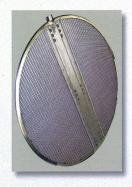
Filter Leaf fabrication is a combination of engineering, experience and technique. Accurately woven filter media, properly engineered drainage chambers and outlet configurations all contribute to a successful product. Our award winning Sani-Leaf design attests to Newark Wire Cloth's success in this field
